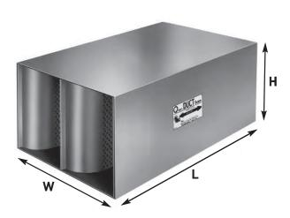
The IAC Type HMS Clean-Flow Quiet-Duct Silencers provide superior performance with mid-range frequency from third thru sixth octave bands and has significant pressure loss for air handling systems requiring a high degree of cleanliness and hygiene. The non-erosive, non-pregnable, "Clean Flow" features make these silencers ideal for hospital, laboratory and clean-room type applications.
