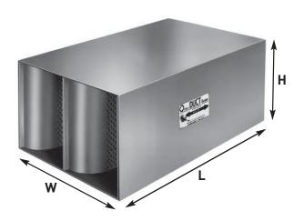
The IAC Type ML Quiet-Duct Silencers provide improved medium-low frequency attenuation as well as low pressure drop aerodynamic performance. When fourth and fifth band performance is critical at the lowest available pressure drop, a Type ML Quiet-Duct selection often results in a shorter silencer length than other equivalent silencer models.
