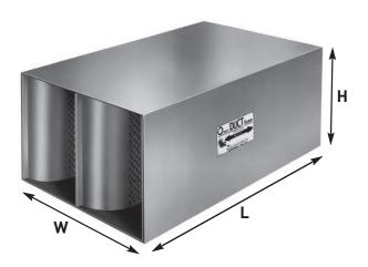
The IAC Type S Quiet-Duct Silencers have been rated with procedures certified in accordance with applicable portions of ASTM E477. All Dynamic Insertion Loss and Self-Noise Acoustic Performance Data were obtained in a NVLAP accredited Aero-Acoustic Laboratory using the duct-to-room reverberant test facility **with air flowing through the silencers.**
