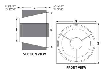
The IAC D-Duct (DDS) Diffuser/Silencer is designed for installation at the outlet of a vane axial fans. Available in sizes matched directly to manufacturer's fan sizes, it has excellent acoustic performance. At the same time it reduces system pressure drop and can be used as an effective inlet cone and silencer. The combined interior diffuser cone and exterior square jacket casing makes these units excellent when requiring aerodynamic-regain devices as well as silencers.
