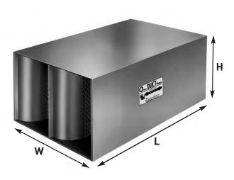
The IAC Type LFS Quiet-Duct Silencers provide superior low frequency attenuation. When low frequencies are controlling, a Type LFS selection often results in a shorter silencer length than the equivalent Type S Quiet-Duct Silencer.
