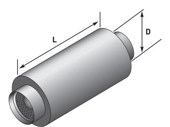
The IAC Type CL Conic-Flow Silencers have been rated with procedures certified in accordance with applicable portions of ASTM E477. All Dynamic Insertion Loss and Self-Noise Acoustic Performance Data were obtained in IAC's Aero-Acoustic Laboratory using the duct-to-room reverberant test facility with air flowing through the silencers.
